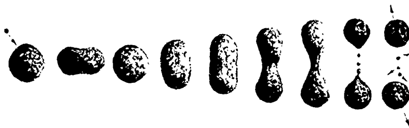
Fig. 24.3 Schematic representation of steps leading to the fission of a compound nucleus, according to the liquid drop model.
